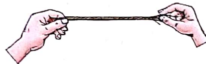
(c) pressing the yarn at one end and scratching the other end
