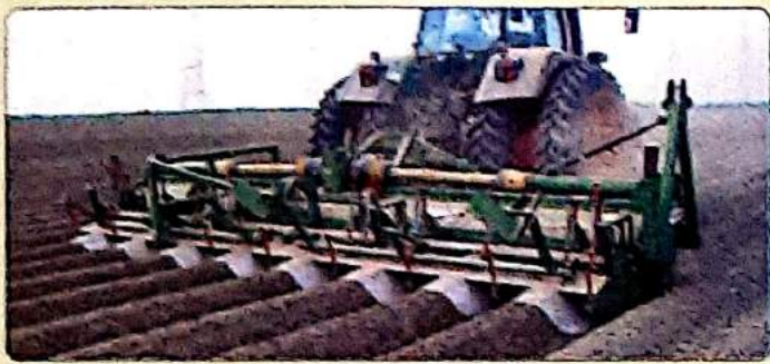
Fig. 1.6 A tractor-driven cultivator
