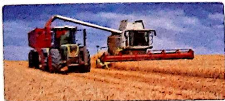
Fig. 1.26 A combine is used for both harvesting and threshing.
