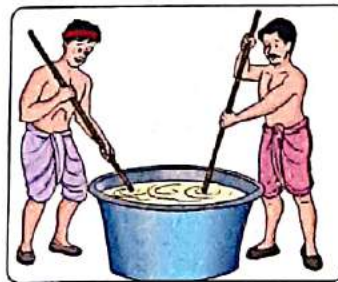
Fig. 3.3 (a) Scouring in tank
